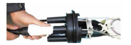
9. Clean the cable surface and ports.
