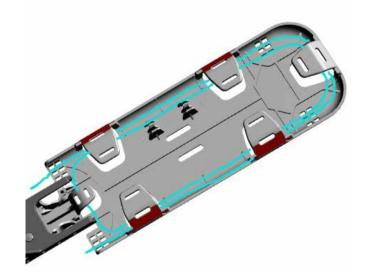
5. Wind the excessive loose buffers in suitable cycles and put in the storage basket.
