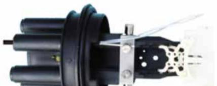
3. Remove the sheath of the cable and clean it.Cut the strengthen member to 5cm length.Put it through the attach screws and bend it to fix on the screw. Then tighten the screw.
